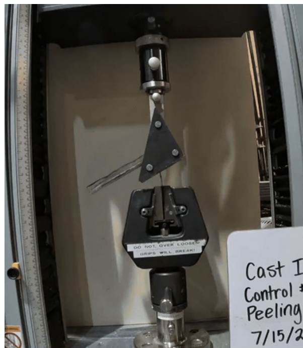
Figure 7.5: Peel test setup including: (a) The original floating roller peel drum setup and dimensions as specified by ASTM D3167 (b) The modified floating roller peel drum test setup
